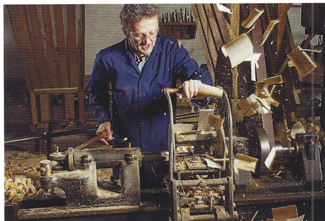
Above: In this photograph, taken shortly before the closure of the mill in 1971, Stott Park's foreman, Jim Graham, is working the hand boring machine to bore holes in blocks of coppice wood
