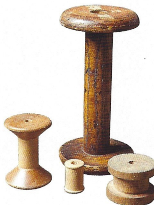
Left: A wide variety of bobbins and reels could be made on the lathes at Stott Park
