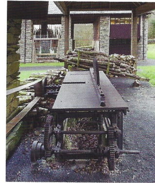
Above: The large circular saw was used to reduce the length of the harvested coppice poles
