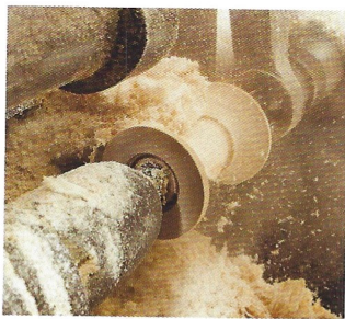
'The bobbin goes to a lathe, where, in turning, it is met by a stout, three-sided sharp tooth or blade, which, quicker than the eye can follow, cuts off the corners and leaves a bobbin, perfect in shape.' Harriet Martineau, Household Words , 1851
